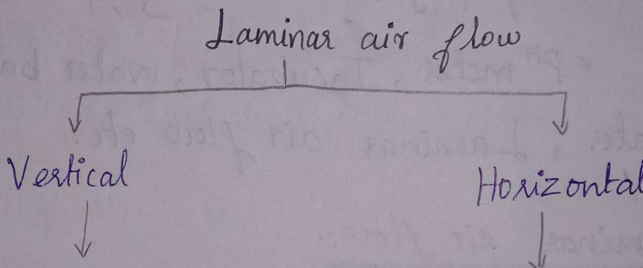
Air moves from Top to Bottom      Air moves from back to the working area to front.
