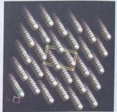
Hexagonal Close Packed (HCP) Structure.
